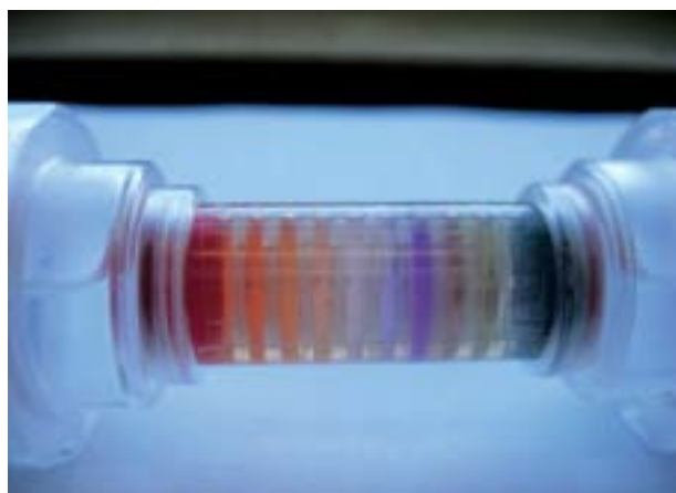
Figure 2. (a) Photograph of the electrolysis cell after the fractionation of the protein digests with the color markers with the pI of 3.9 (orange) and 5.3 (purple). (Bottom left) peptide autofocusing; the yellowish color, in the compartment on the left of the purple zone, corresponds to the impurity in the pI marker with higher pI value. (Upper right) the same sample focused in 2% ampholyte solution. (Middle right) autofocused fractions in the harvesting vessel. The bubbles trapped inside the compartments result from the manual handling of the chamber. No dependence of the amount of air bubbles on the mode of operation was observed. (b) Plot of the pH values measured in the collected fractions.
