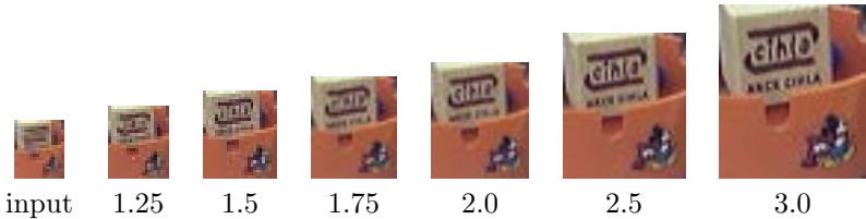
Figure 6: Superresolution with non-integer factors of short-exposure images. The first left image is one of ten low-resolution frames acquired by a webcam that were used to estimate high-resolution images. The proposed method was run with different superresolution factors from 1.25 to 3. The estimated HR images appear in their original size.
