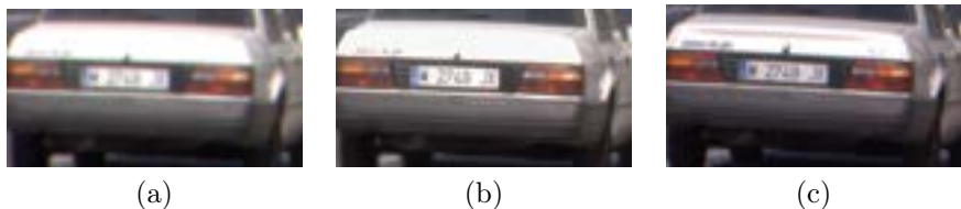
Figure 5: Superresolution of images acquired with a digital camera: Several low-resolution images were acquired with the digital camera and superresolution has been applied. (a) bilinear interpolation of one low-resolution image, (b) result of the proposed superresolution algorithm, (c) image taken by the same camera but with optical zoom. The proposed algorithm achieves reconstruction comparable to the image with optical zoom.
