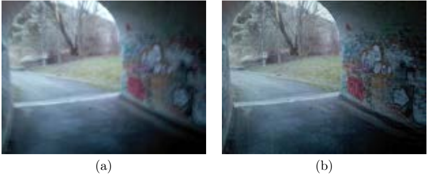
Figure 9: Smartphone deconvolution application: (a) image acquired with the phone and blurred due to camera shake, (b) sharp image estimated by the deconvolution algorithm running on the phone using prior information about camera motion from phone gyroscopes.
