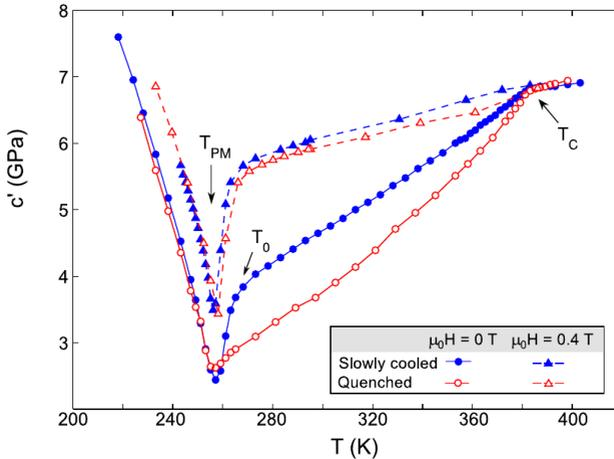
**Figure 10:** Summary of results of papers [B1] and [B2]:  $c'(T)$  softening curves upon cooling with and without external magnetic field. Results for two materials are shown; the quenched material has higher density of defects, which increases the magnetoelastic coupling effects.  $T_C$  and  $T_{PM}$  denote the Curie point and the premartensitic transition temperature, respectively.
