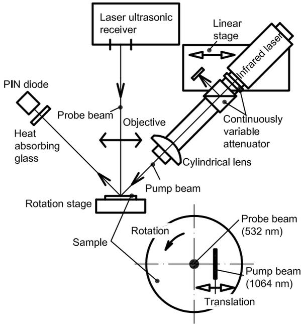
**Figure 4:** A schematic sketch of the line-source/point-receiver LU setup. Modified after [51].
