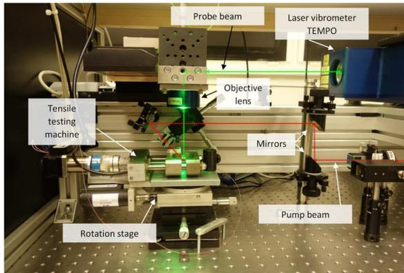
**Figure 5:** The experimental arrangement for line-source/point-receiver measurements under uniaxial stress. Modified after [53]. Photograph by J. Zidek.
