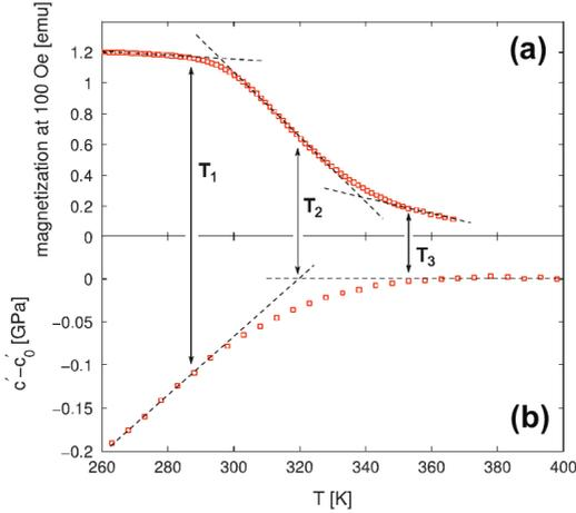
**Figure 11:** Temperature evolutions of the magnetization (a) and soft shear elastic modulus  $c'$  for the CoNiAl ferromagnetic shape memory alloy. In (b),  $c'_0$  stands for the  $c'$  coefficient unaffected by magnetoelastic softening, i.e. having the  $dc'/dT$  slope given solely by phonon-mediated softening.
