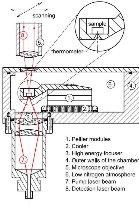
**Figure 1:** Schematic sketch of the temperature chamber used for the modal RUS measurements
