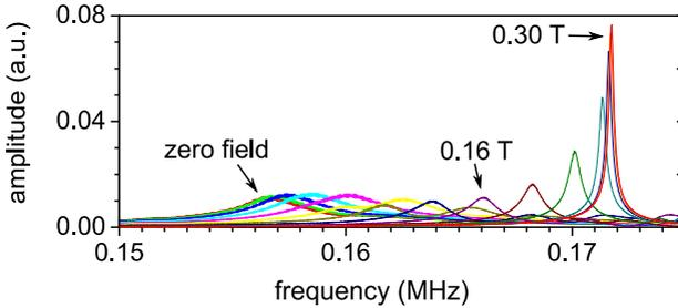
**Figure 9:** Evolution of a chosen resonant peak in RUS measurement with increasing external field (modified after [74]). The field suppresses the rotations of the magnetization vector, which leads to stiffening (i.e., increase of the resonant frequency) and decrease of magnetoelastic damping (i.e. decrease of the peak width). The shown example was measured on Ni-Mn-Ga premartensite at 240 K.
