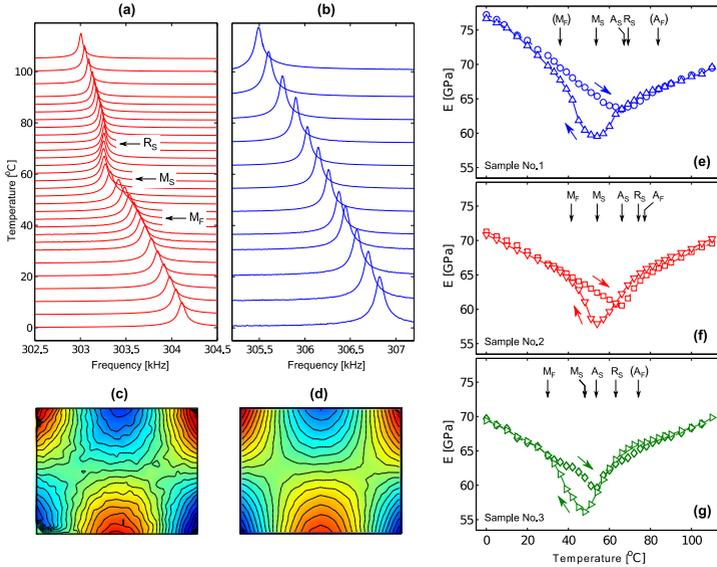
**Figure 6:** A summary of results of paper [A1]: (a,b) temperature evolutions of a chosen RUS resonant peak with and without the film; (c,d) the corresponding modal shapes; (e,f,g) resulting evolutions of Young's modulus for three different films. The labels  $(A, R, M)_{(S,F)}$  refer to start and finish temperatures for austenite, R-phase and martensite, respectively.
