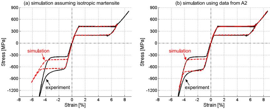
**Figure 7:** A comparison of the simulation and experiment for unidirectional tension/compression tests of polycrystalline NiTi using the constitutive model described in [67]: (a) simulation assuming isotropic elastic constants for polycrystalline martensite; (b) simulation assuming anisotropic elasticity of martensite developing with reorientation, as described in [A2]. Graphs courtesy of P. Sedláč.
