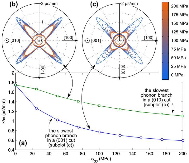
**Figure 8:** Evolutions of soft acoustic phonons (slowest transversal acoustic modes) for the Fe-Pd single crystal studied in [A3]. As seen in (a), both phonons exhibit decrease in slowness, which means stiffening. Polar plots of the slowness curves in two principal cuts are seen in (b) and (c). Modified after [A3].
