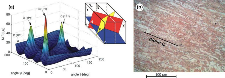
**Figure 13:** Symmetry class determination based on elastic constants for fine-grained polycrystalline copper: (a) a function measuring the level of mirror symmetry of elastic properties over a plane with a normal vector given by Euler angles  $\psi$  and  $\theta$ ; (b) optical microscopy of the microstructure showing significant grain elongation along the plane identified in (a). Modified after [D1].
