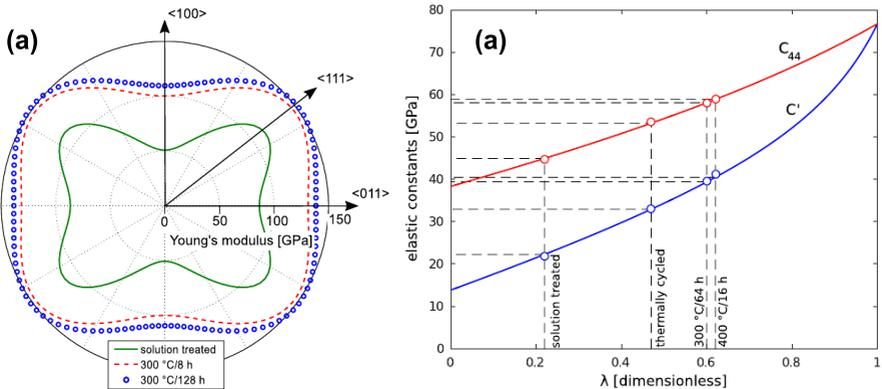
**Figure 12:** Main results of papers [C2] and [C3]: (a) the effects of  $\omega$ -particles growth on anisotropy and magnitude of Young's modulus of Timetal LCB single crystals; (b) the same effect on shear elastic moduli of Ti-15Mo single crystals. In both cases, the growth leads to strong stiffening and isotropization.
