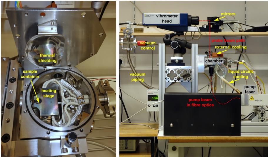
**Figure 3:** The vacuum chamber for high-temperature measurements (on the left) and the experimental setup for single-point RUS measurements using this chamber (on the right). The optical paths of the pump and probe lasers are outlined by dashed red lines. Photograph by J. Zidek.
