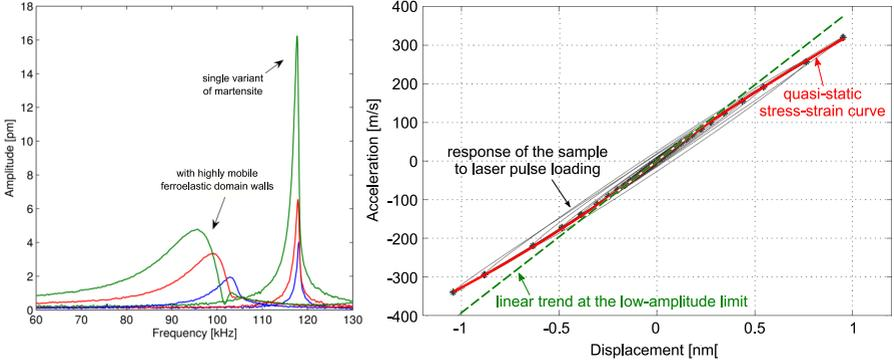
**Figure 17:** Nonlinear stress-strain character of a Ni-Mn-Ga FSMA single crystal in the martensite phase. On the left: difference in RUS spectra with and without the highly mobile ferroelastic domain walls, different colors refer to different pump beam amplitudes. On the right: the stress-strain curve estimated from the RUS measurements. Modified after [102].
