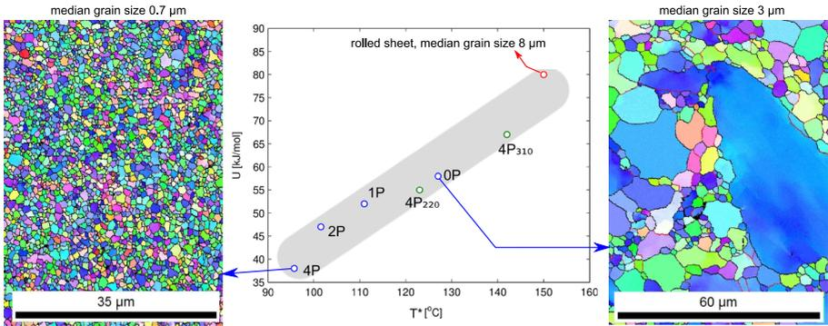
**Figure 14:** Correlation between activation energy  $U$  and onset temperature  $T^*$  for GB sliding in the AZ31 alloy revealed by ultrasonic measurements. Individual points in the graph represent samples with different levels of grain refinement, for the smallest (4P) and largest (0P) grains, EBSD maps of the microstructure are given. Modified after [D2].
