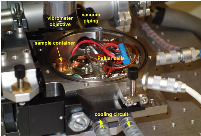
**Figure 2:** Detail of the temperature chamber for modal RUS measurements. Photograph by J. Zídek.
