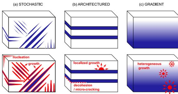
**Figure 16:** Types of heterogeneities (upper row) and the thermally activated processes in them (lower row) to be studied in the current research project lead by the applicant.
