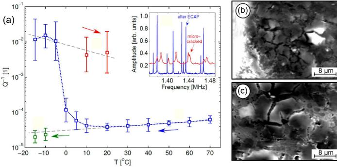
**Figure 15:** Detection of surface micro-cracking of finely grained AZ31: (a) an evolution of RUS spectra along a temperature cycle; (b,c) micro-cracked regions along the edges of the sample. The green experimental points in the lower left corner of (a) were obtained for a sample with a special surface treatment that prevented micro-cracking. Modified after [97].
