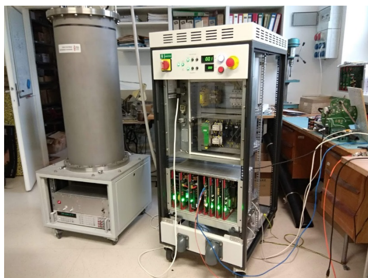
Fig. 6 Precise 100 kV supply for FEG (right) and reference divider (left) during testing in our lab.
